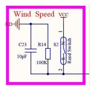
According to the times of the reed switch is turned on to calculate the wind speed.
